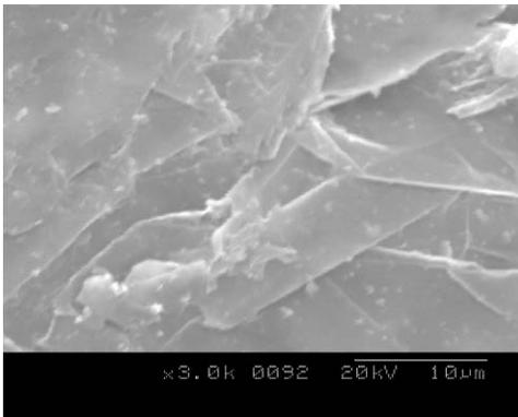
Figure 2. SEM of epoxy-expanded graphite-carbon black composite
