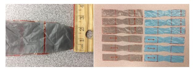
Figure 1: Folded rectangle sample with center cut to 2cm Figure 2: Example of samples cut to 2cm gauge
