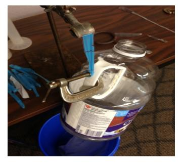
Figure 3: Note the set up, and that the sample is folded under the clamp.
