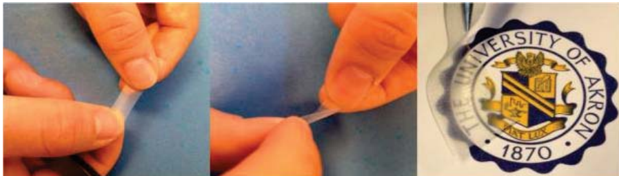
Figure. Solvent free polymer electrolyte membrane fabricated by photo-curing a 28/42/30 PEGDA/SCN/LiTFSI mixture. This self standing film is light weight, transparent, and flexible which can be stretched, bended or twisted, and molded in any forms. Its room temperature ionic conductivity is on the order of E-3 S/cm that reaches E-2 S/cm at elevated temperatures above 50 C.
